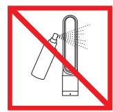
Do not spray scented products such as air freshener or perfume near the filter or the appliance.
